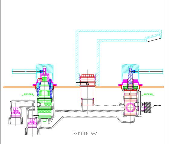
OMNIA: A high flow rim mount thermostatic valve ideal for Nursing home, Hospital, Hotel and residential Home, now like never before the entire whirlpool piping system including the pump can be disinfected cleaned and rinsed in 5 minutes or less without wasting time, water and energy
