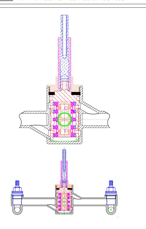
THE ESATA DIVERTER CARTRIDGE IS PATENTED PROTECTED IN ALL NORTH AMERICAN MARKET. THE DIVERTER CARTRIDGE IT HAS AN INTEGRAL PRESSURE BALANCE SPOOL TYPE SPECIFICALLY MADE FOR THE OLD FASHION 3 HANDLE WALL MOUNTED FITTING. IT IS THE FIRST FITTING WITH AN INTEGRAL HIGH LIMIT DEVISE THAT COMPLY TO ASSE 1016 STANDARD
